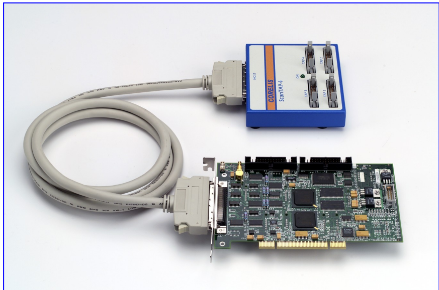
Figure 1. PCI-1149.1/Turbo Boundary-Scan Controller
