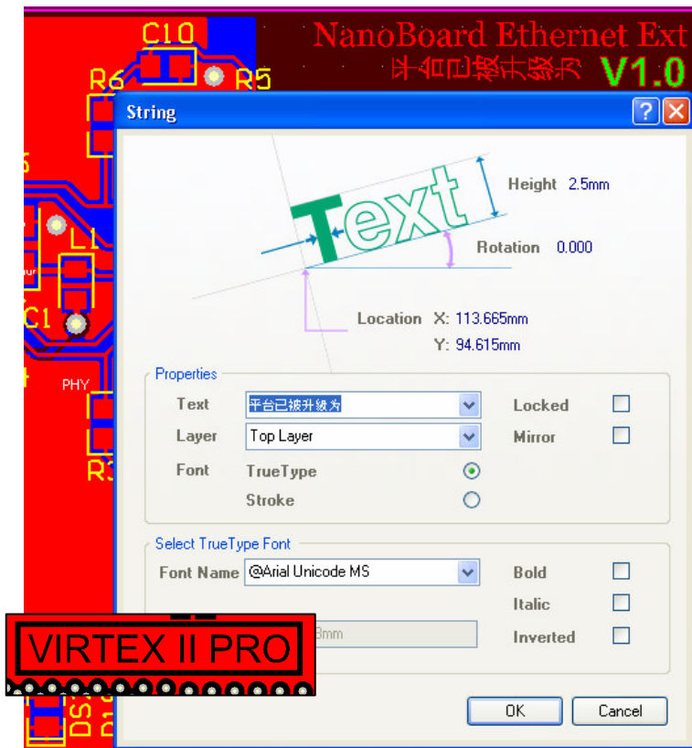
Figure 11. Use the new TrueType font support to display text in your preferred font face. Invert the string if you need it etched in a copper layer.
