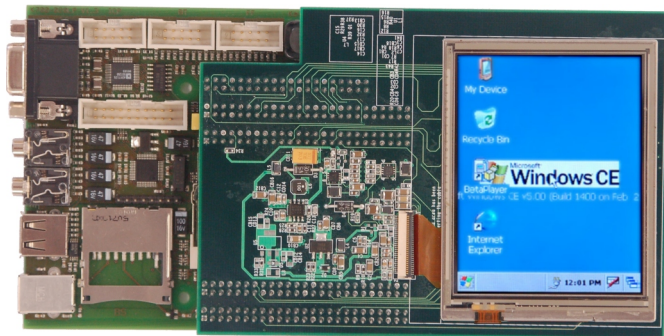
TRITON Starter Kit baseboard with optional MI Board and QVGA touch screen display mounted
